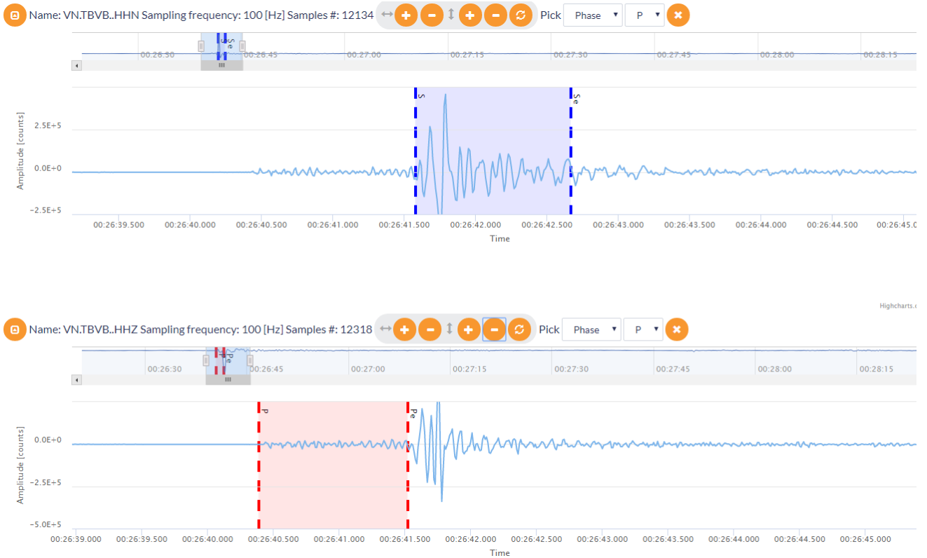
Figure 2. Phase picking demonstration for S (upper frame) and P (lower frame) waves.
